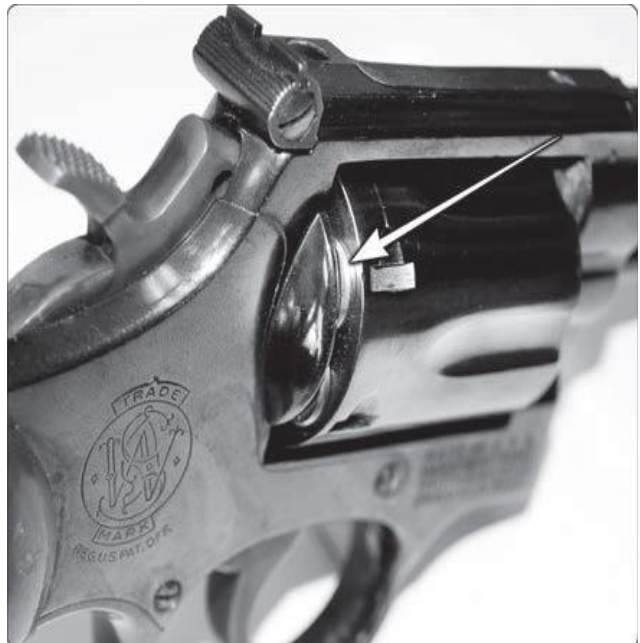
(Figure 6-2) Cylinder placement with partial load
